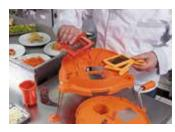
Remove the grids and install the new ones, replace the blade under the bottom part.
